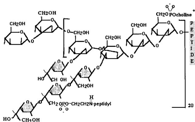
FIG. 1. Diagram of pPGalMan. The mannopyranosyl residues in each tetrasaccharide are attached by  $\alpha$ -1,2 linkages and the tetrasaccharides are attached by  $\alpha$ -1,6 linkages. The mannan is attached to the peptide by an *O*-glycosidic linkage to a seryl residue. Manno-oligosaccharides are attached to seryl and threonyl residues. An average of one galactan chain branches from each manno-octasaccharide and one phosphocholine phosphodiester is attached to C-6 of a mannopyranosyl residue.
