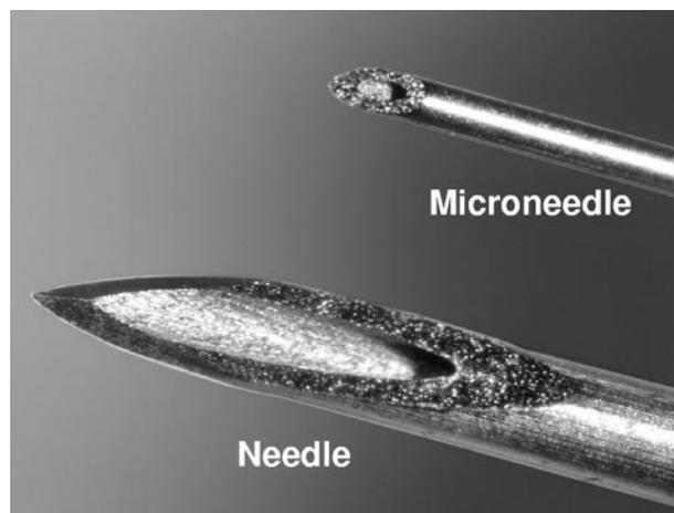
FIG. 1. Comparison of standard 27-Ga needle to 34-Ga microneedle. The displayed microneedle has an inner diameter of 76  $\mu$ m, an outer diameter of 178  $\mu$ m, and a total exposed length of 1.0 mm.
